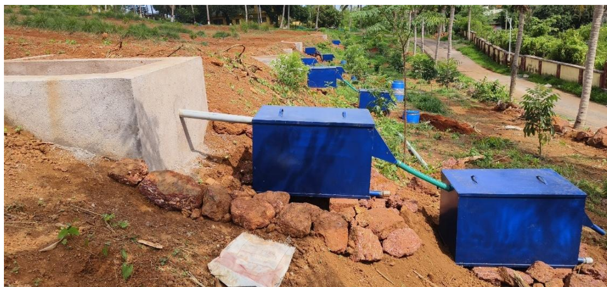
Multi-slot devices installed to record the run-off data in cashew based agroforestry system
